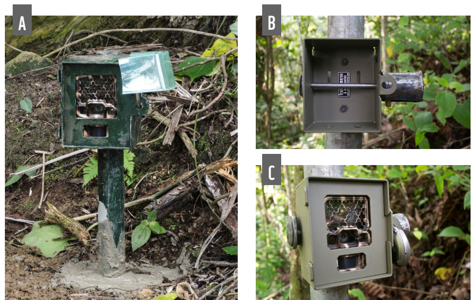
Figure 10-8. Using custom-made security posts for the highest protection when deployment in high-risk areas is unavoidable. The camera trap is secured within a steel box and bolted or welded onto a steel post, which is then sunk into the ground and fixed with concrete ( A ). The plastic tub is a rain cover for the padlock. If the camera trap is designed to be compatible with a cable lock, it can also be secured within the box by passing a metal skewer through the camera trap's casing ( B ). In combination with the padlock on the outside of the box, the camera is then doubly-secured ( C ).
