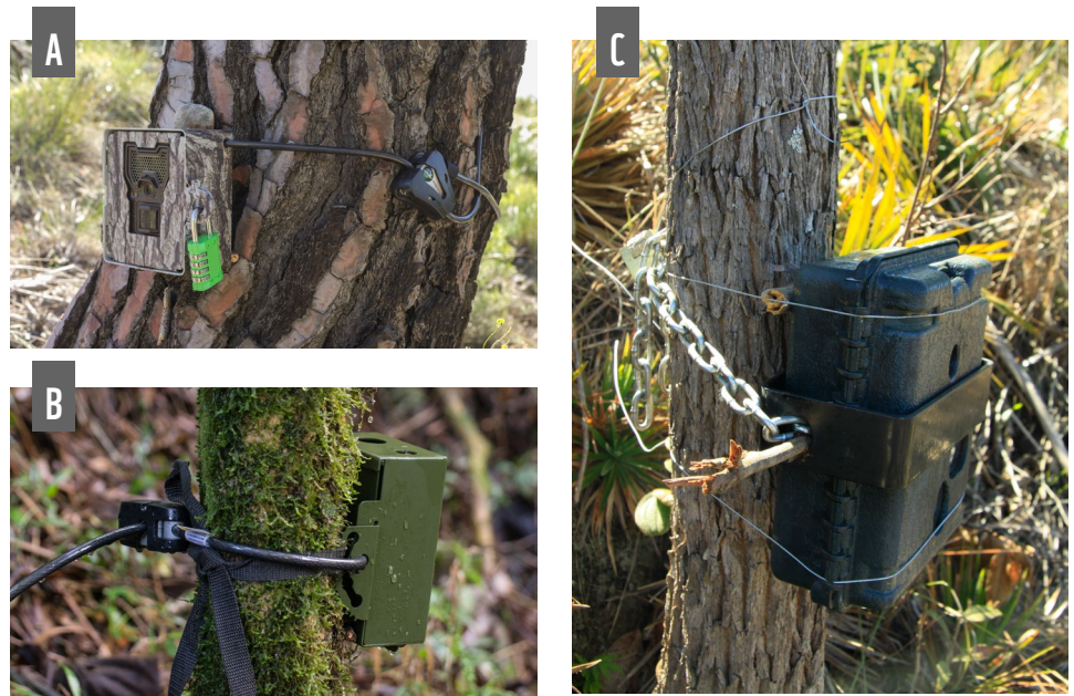
Figure 10-7. Using cable locks ( A and B ) and chains ( C , © Guilherme Ferreira) to secure camera traps in the field and deter thieves.
