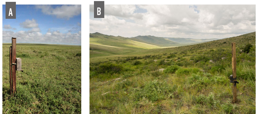
Figure 10-2. Fixing camera traps in the environment when trees are unavailable. In the Serengeti plains, metal posts and steel security boxes were used to help guard against attacks from elephants and hyenas ( A , from Swanson et al. 2015). In Mongolian steppe habitat, wooden stakes hammered into the ground were sufficient for mounting cameras in the environment ( B ).
