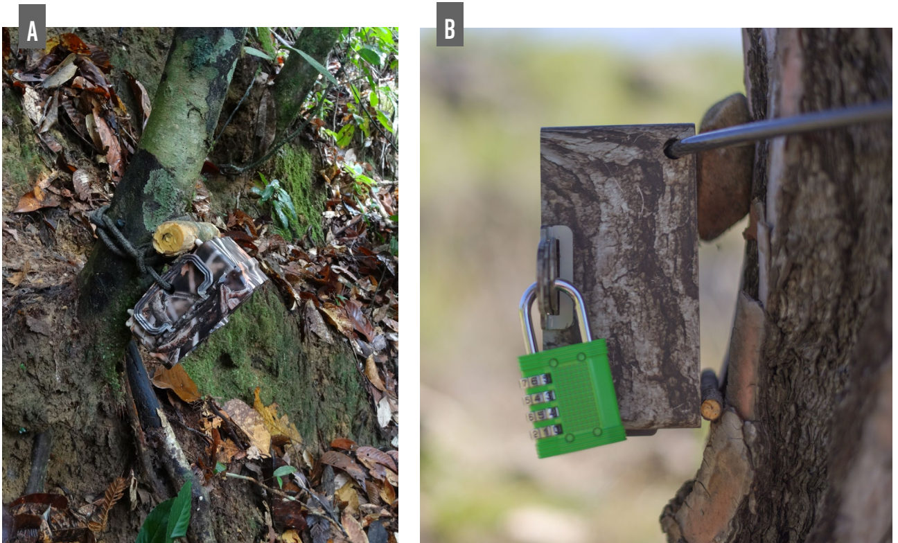
Figure 10-4. Making fine adjustments to the aim of a camera trap. In steep areas it will often be necessary to angle your camera downwards or upwards to run parallel with the ground surface. If you are not using a dedicated camera mount, short sections of wood, wedged behind the camera trap, are an effective and low-cost alternative (A). If you are using trees or other natural objects to mount your camera traps, it will often be necessary to make fine adjustments to the angle, even if the terrain is relatively flat (B). Again, short pieces of wood or rock, firmly wedged behind the camera, can be used.
