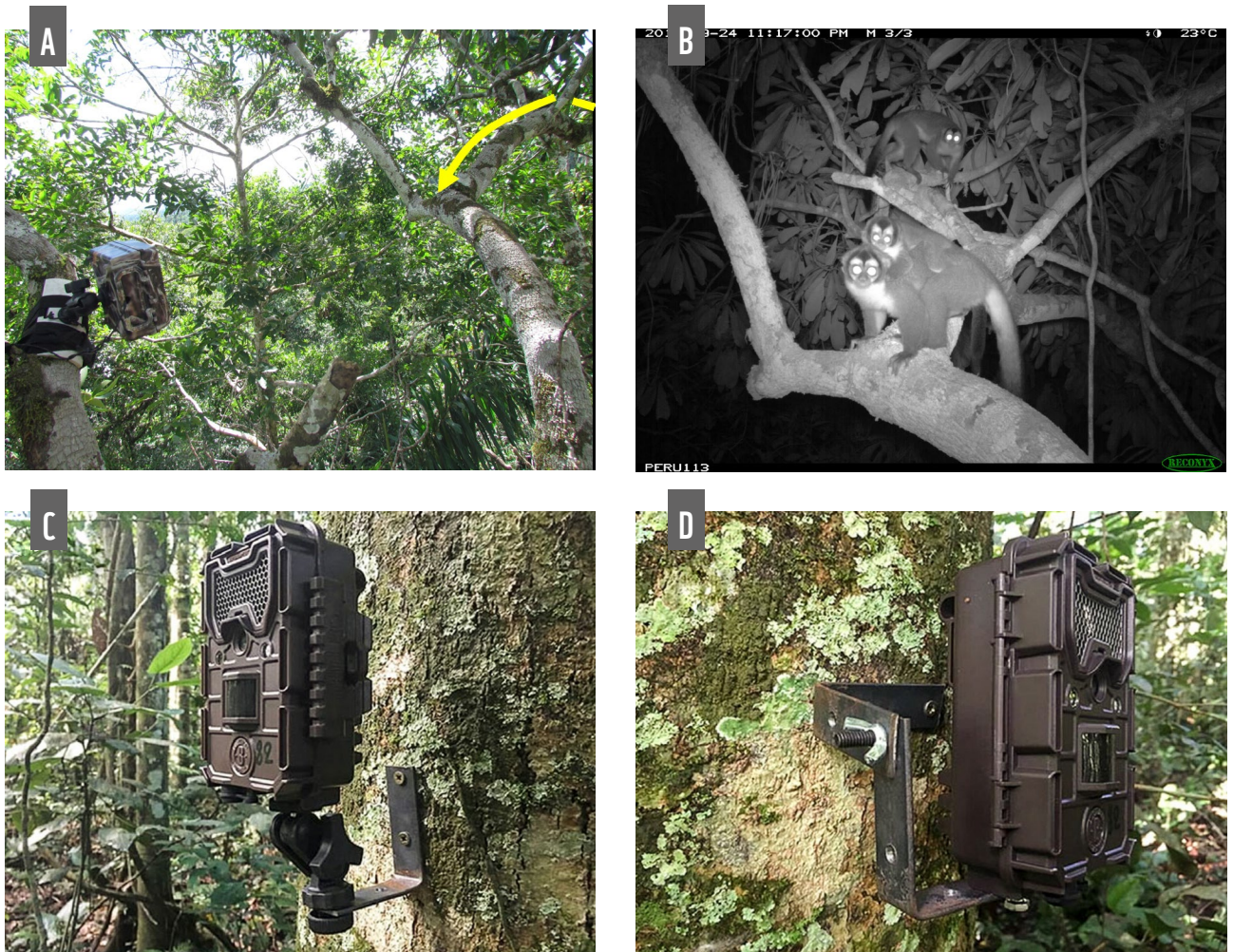
Figure 10-11. Arboreal camera trap deployment. Cameras should be fixed near to the trunk of the tree to minimise movement from wind and are most effective if aimed at large branches (A). The field of view of the camera trap in A is shown in B. Camera traps can record rare behaviours of species, such as Aotus nigriceps , which are difficult to otherwise monitor (B). Cameras can be fixed in the canopy using ball head (C) or L-bracket (D) mounts. Images © Tremaine Gregory (A and B) and © Mark Bowler (C and D).
